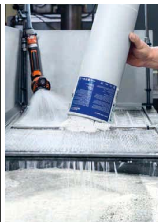
At BRITA, the ion exchange resin is regenerated at the company's own plant and subsequently reused in new filter cartridges.
